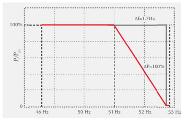
/ Frequency droop function of Fronius inverters with MicroGrid setup. Fully adjustable to harmonise perfectly with the Inverter-Charger.
